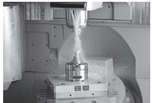
hs dock mandrel actuating unit in use
