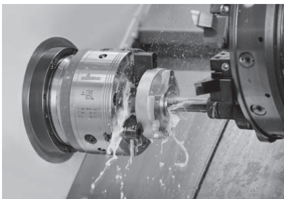
B-Top jaw chuck in use
