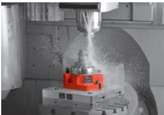
ms dock mandrel actuating unit in use
