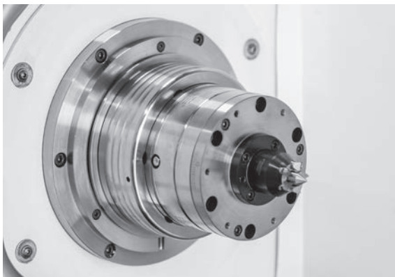
Face driver adaptation on the machine
