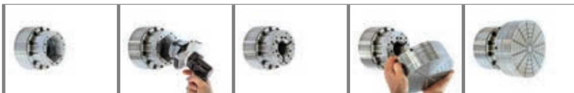
Remove clamping head Insert magnet module Clamping device with clamping head Insert magnet module Clamping device set-up
