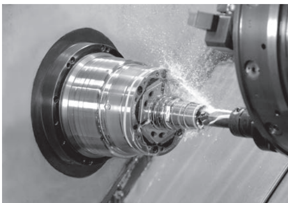
TOPlus combi pull-back chuck in use
