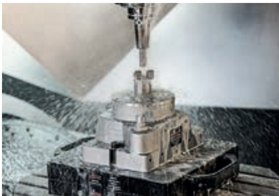
MANOK plus manual stationary chuck in use
