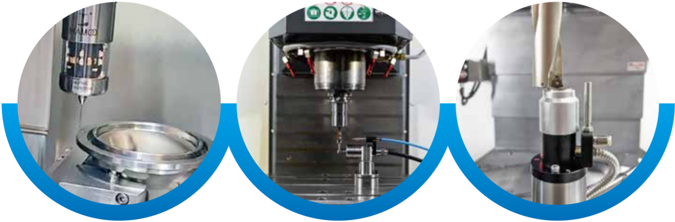
Vertical Lathe and Rotary Center Measurement Applications Machining Center Tool Diameter and Tool Length Measurement, and Broken Tool Detection Economical Tool Setter for Tool Length Setting and Broken Tool Detection
